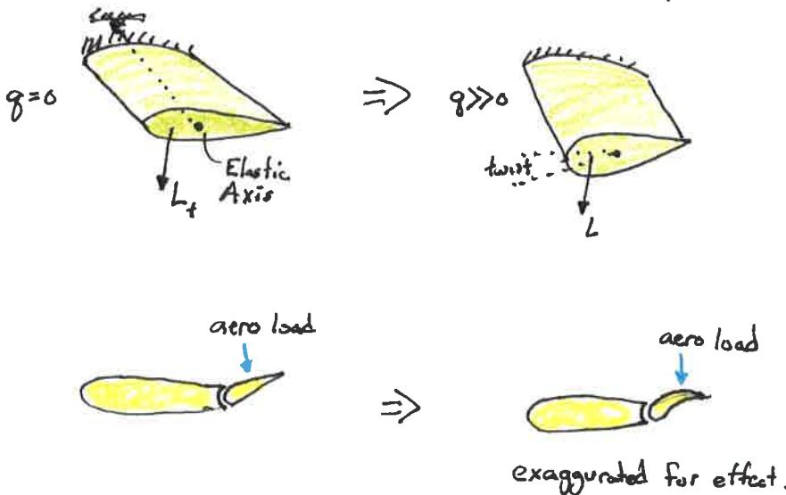
For light aircraft, the static margin even in an incompressible flow may strongly depend on the flight velocity
