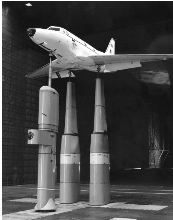
Fig. 47. Full-scale T-39 in test section of 80 ft \times 120 ft facility of the NFAC (photo courtesy of the NASA Ames Research Center).
