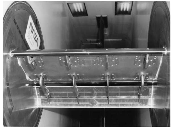
Fig. 44. Multi-element airfoil model mounted in the LTPT test section (photo courtesy of the NASA Langley Research Center).
