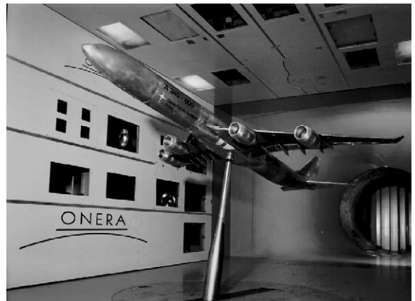
Fig. 50. Full model of A340-600 in test section of ONERA F1 facility (photo courtesy of ONERA).
