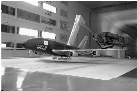
Fig. 46. Full model of A3XX during ground effect testing in DNW-LLF (photo courtesy of DNW).
