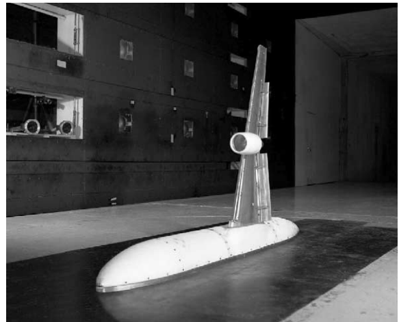
Fig. 45. Semispan EET model as tested with 2D standoff in the 14 ft \times 22 ft tunnel (photo courtesy of the NASA Langley Research Center).
