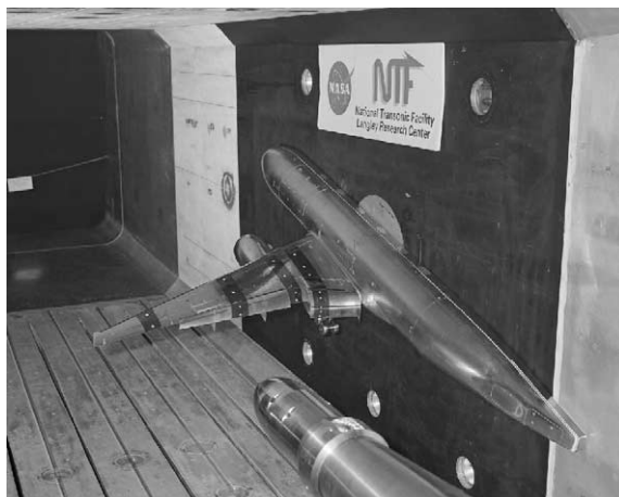
Fig. 51. Semispan model of B777-200 mounted in the NTF test section (photo courtesy of the NASA Langley Research Center).
