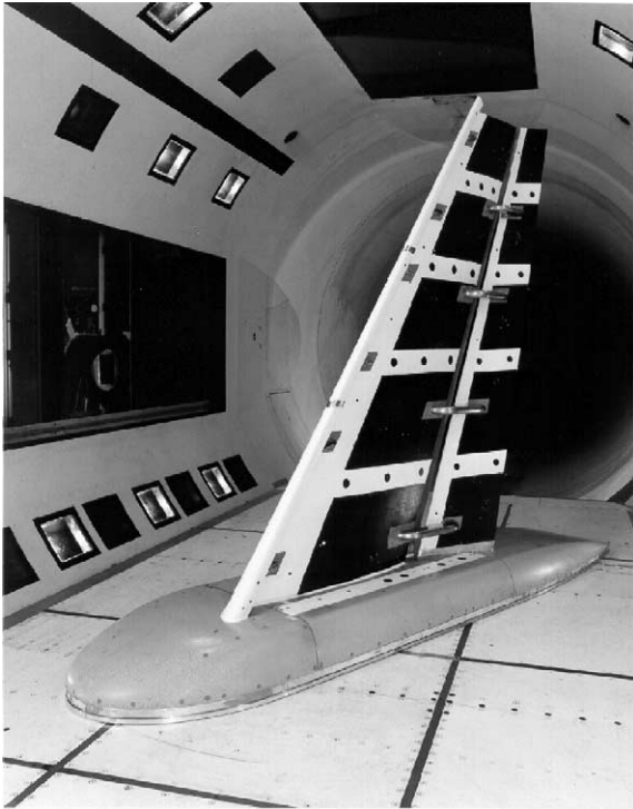
Fig. 48. Trapezoidal wing model with full-span slat and flap mounted in the 12 ft PWT (photo courtesy of NASA).
