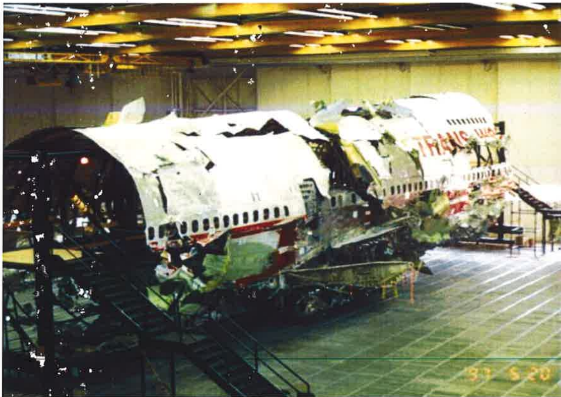
Figure 29. A photograph of the right side of the large three-dimensional reconstruction, with the support scaffolding visible.
