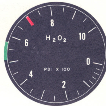
APU HYDROGEN PEROXIDE TANK PRESSURE GAGE
