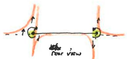
The velocity at the wing tip is infinite!
