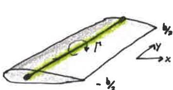
$$C_L = \int C_\theta dy = \int_{-b/2}^{b/2} \frac{2R}{z} \quad \underline{\text{Finite!}} \quad \underline{\text{Wrong!}}$$
