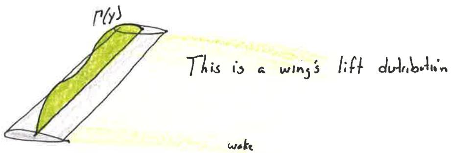
$$C_L = \int_{-b/2}^{b/2} C_e(y) dy \quad \text{also} \quad L = \int_{-b/2}^{b/2} L' dy = \int_{-b/2}^{b/2} \rho V_\infty \Gamma(y) dy$$
