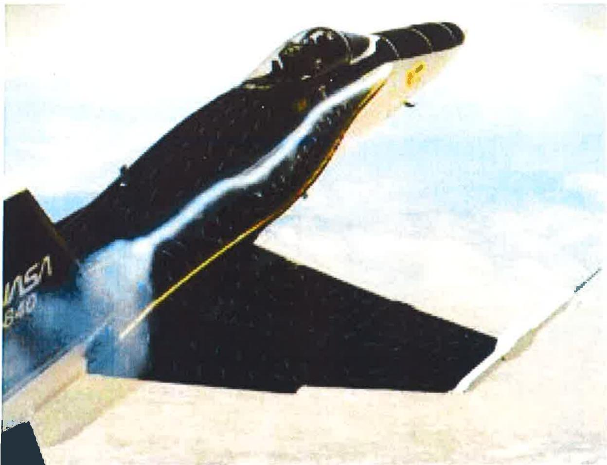
The F-18 had a significant development issue with the LEX stroke vortex bursting and interacting with the canted verticles. The vortex created large stresses and eventually fatigue issues.
