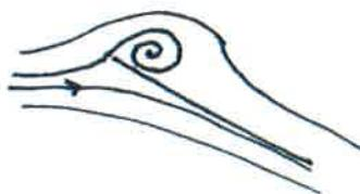
Vortex lift is produced from the leading edge suction
