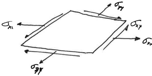
No traction in z means  $\sigma_{zz} = 0$ . Take initial Hookean strain-stress equation
