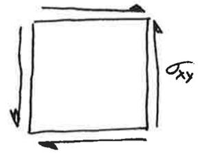
The stress state is  $\sigma = \begin{bmatrix} 0 & \sigma_{xy} & 0 \\ \sigma_{xy} & 0 & 0 \\ 0 & 0 & 0 \end{bmatrix}$ . The strain state is  $\epsilon_{xy} = \frac{1}{G} \sigma_{xy}$
