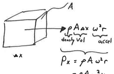
$$\textcircled{1} \quad \frac{dp}{dx} = -p_x = -\rho A \omega^2 x \quad \text{integrate } \int dp = \int -\rho A \omega^2 x \, dx$$
