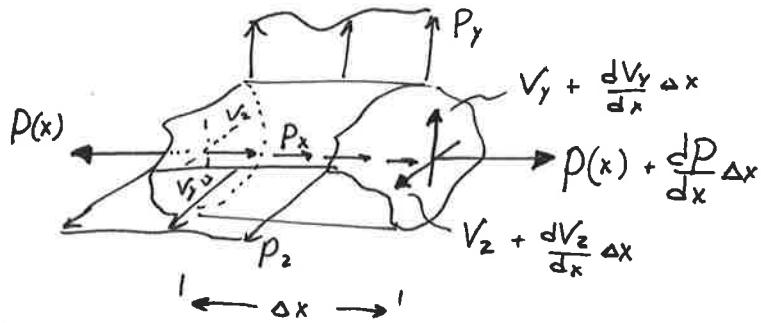
$$\sum F_x = 0 = \underbrace{-P(x)}_{\text{left}} + \underbrace{P(x) + \frac{dP}{dx} \Delta x}_{\text{right}} + \underbrace{P_x \Delta x}_{\text{internal force}} \Rightarrow \frac{dP}{dx} + P_x = 0$$
