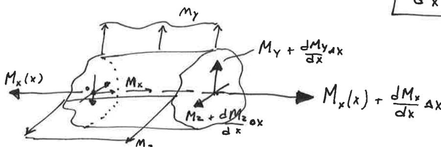
$$\sum M_x = 0 = -M_x + M_x + \frac{dM_x}{dx} \Delta x + M_x \Delta x \Rightarrow \frac{dM_x}{dx} = -M_x$$
