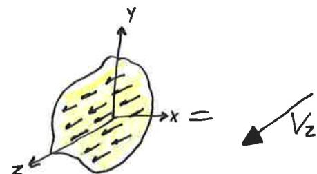
Moment "F.d" force times distance  $\equiv$  integral of stress times distance over an area.
