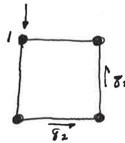
$$\sum M_{x_1} = 0 = \underbrace{q_2 \cdot 10^{\text{in}}}_{\text{force}} \cdot \underbrace{10^{\text{in}}}_{\text{distance}} + q_3 \cdot 10^{\text{in}} \cdot 10^{\text{in}}$$
