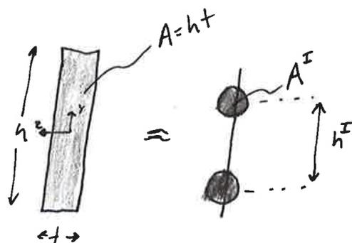
Can we find  $A^I$  and  $h^I$  such that the areas are identical and the moments of inertia are identical? Yes.
