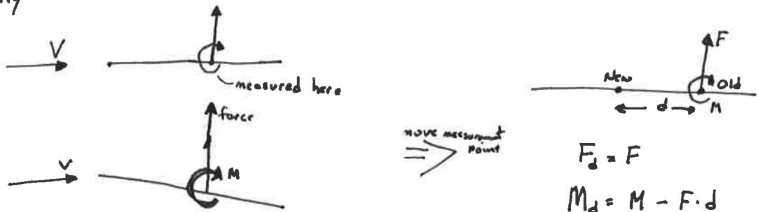
If the moment increases with force, where can we move the measurement point such that the increase in  $M$  wrt  $L$  decreases?
