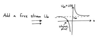
As we approach the point source, the flow velocity decreases to a stagnation point. Aft of the source, the flow velocity decreases from a higher velocity back to freestrom.
