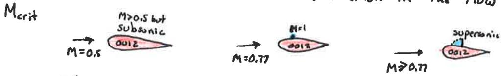
The critical Mach number for an NACA 0012 is  $M 0.77$ .
