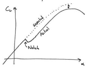
Aero engineers don't like notches since they (the notches) reduce Chmax by the notch width (approximately). And, the notch can generate non-linear flight behavior. And, notches can annoy or increase pilot workland or stress.
