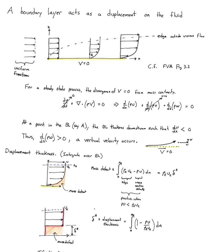
If the flow were uniformly at velocity us and density pe, what height St is necessary to give the mass defect seen in the BL.
