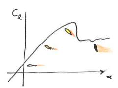
The art of high lift is the art of delaying, mitigating or eliminating Separation while maximizing Circulation.
