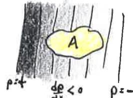
$$\Delta C_d^{\text{buoyancy}} = \frac{\Delta D'_{\text{buoyancy}}}{\frac{1}{2} \rho V_{\infty}^2 c} = \frac{\pi}{6} \frac{A}{h^2} C_d$$
