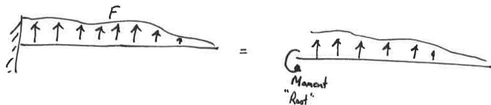
Let's match the total lift and the bending moment and allow span and lift distribution to vary. What is the optimal lift distribution?
