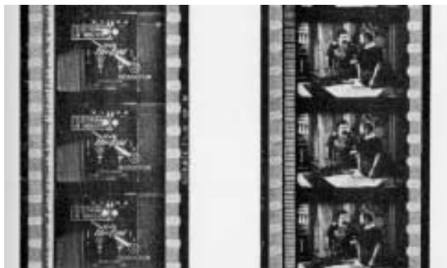
Figure 1: Variable Area and Variable Density Sound Tracks (from Moir)
